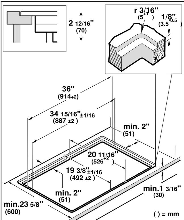
**Flush installation:** The appliance can be installed in the following temperature- and water-resistant countertops:
