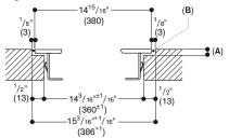
**A**: <sup>1</sup>/<sub>B</sub>" (3.5<sup>-0,5</sup>) **B**: Fill with silicone
