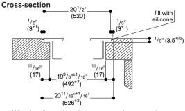
When installing with appliance cover or adjustment strip, pay attention to the deeper cut-out and the front and rear groove width.
