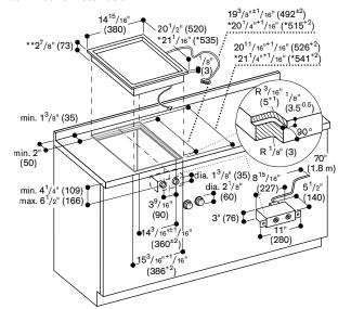
$^\star$  With appliance cover or adjustment strip. See separate planning notes on page 77. \*\*  $31\!/\!2^*$  (88) in the area of the cable clip (right, center).
