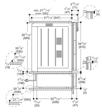
Side view of WS 482 below BS Combi-steam oven, BM Combimicrowave oven or CM espresso machine
