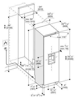
The door face dimensions are designed for a maximum gap of % " (3 mm). See more details on page 252.
