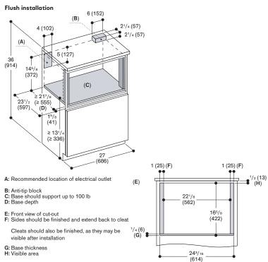
If under a counter, minimum clearance to counter top
