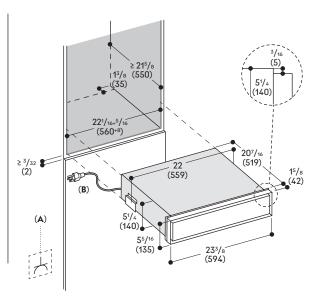
A: Accessible electrical connection B: Fixed cable
