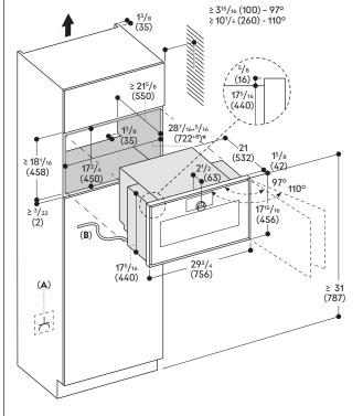
A: Accessible electrical connection B:Fixed cable
