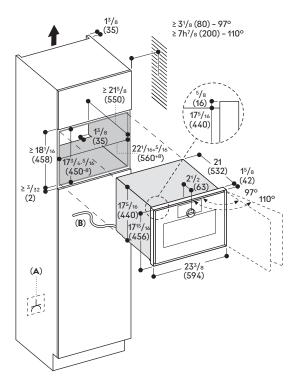
A: Accessible electrical connection B:Fixed cable
