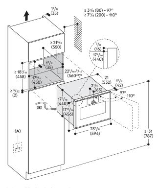
A: Accessible electrical connection B:Fixed cable
