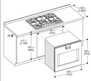
A: Min. countertop thickness 3/4" (20 mm) for surface mounted installation
