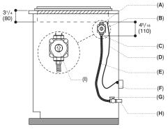
A: 3/6" (9.5 mm) NPT B: Gas regulator C: 1/2" (12.7 mm) NPT D: Power cable 4" (100 mm) E: Flexible gas line F: 120 V socket
