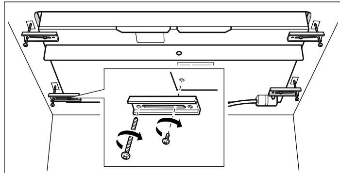
The appliance must be secured from below using the hold-down brackets provided, so it does not slip.
