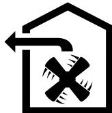
The air which is drawn in is cleaned by the grease filters and conveyed to the exterior by a pipe system.
