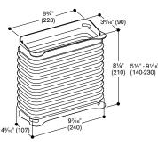
AD 851 041: Connecting piece VL 200 for extension with flat duct DN 150 for extra deep countertop
