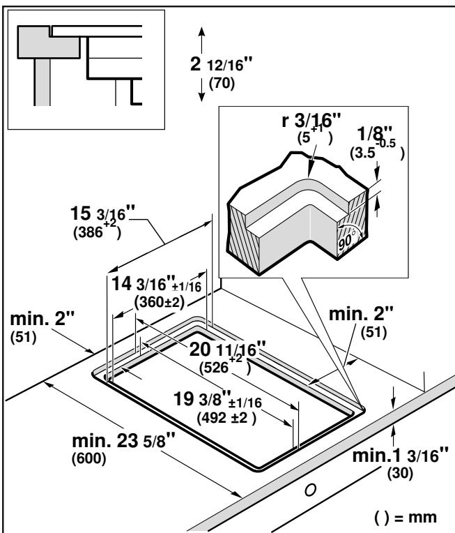
**Flush installation:** The appliance can be installed in the following temperature- and water-resistant countertops:
