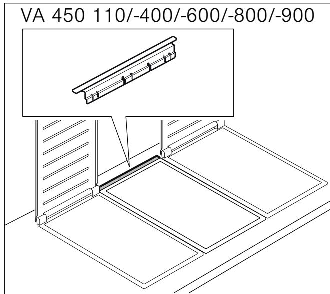
**Combination with appliance cover:** The appliance cover VA 440 010 is available separately as a special accessory. When creating the cut-out, bear in mind the additional space required for the appliance cover.
