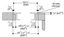
When installing with appliance cover, pay attention to the deeper cut-out and the front and rear groove width.
