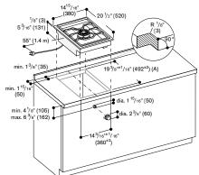
(A) When installing with appliance cover, take the deeper cut-out into consideration (observe separate planning notes) See separate planning notes on page 113.
