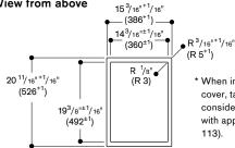
\* When installing with appliance cover, take the deeper cut-out into consideration. See "Installation with appliance cover" on page 113).
