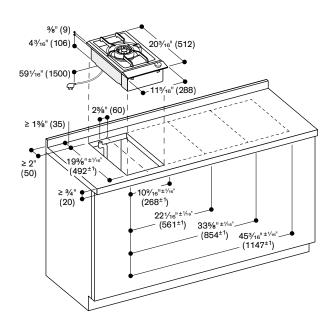
Minimum distance from the appliance cut-out to the side wall  $11^{13}/16$ " (300 mm).
