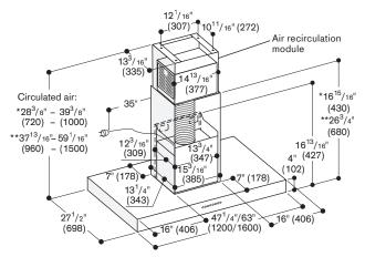
\* With the air recirculation duct cover AD 442 116 suitable for ceiling heights of 7'9" (2.35 m) to 8'6" (2.60 m).
