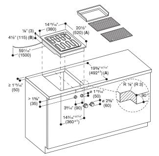
Minimum countertop thickness %'' (20 mm) for surface mounted installation. See separate planning notes on page 104.
