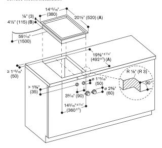
Minimum countertop thickness %'' (20 mm) for surface mounted installation. See separate planning notes on page 104.
