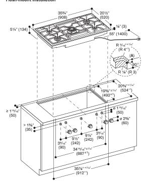
Minimum countertop thickness 1  $^3\!\!/\!\!\omega''$  (30 mm) for flush installation. See separate planning notes on page 106.
