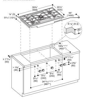
Minimum countertop thickness %'' (20 mm) for surface mounted installation. See separate planning notes on page 104.
