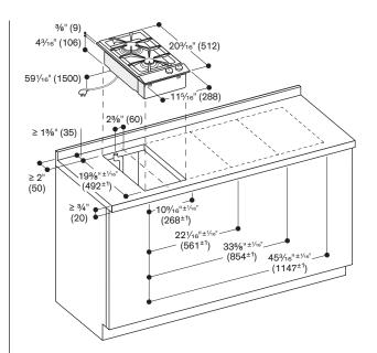
Minimum distance from the appliance cut-out to the side wall 11<sup>13</sup>/<sub>16</sub>" (300 mm).
