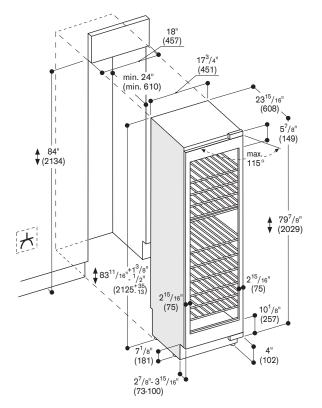
The door face dimensions are designed for a maximum gap of  $^{\prime}\!\!\!/_{8}$  " (3 mm). See more details on page 252.
