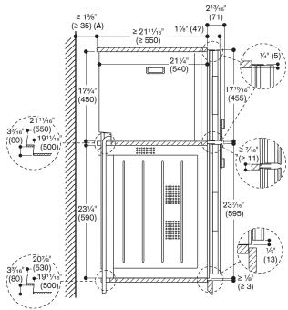
A: Only required if the water hoses for the BS steam oven cannot be accommodated in the corner recesses of the appliances.
