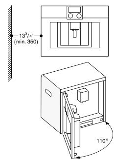
If using the 92° door hinge restrictor (spare part no. 00636455), the minimum distance to the wall is only  $3^{15}/16^{\circ}$  (100 mm).
