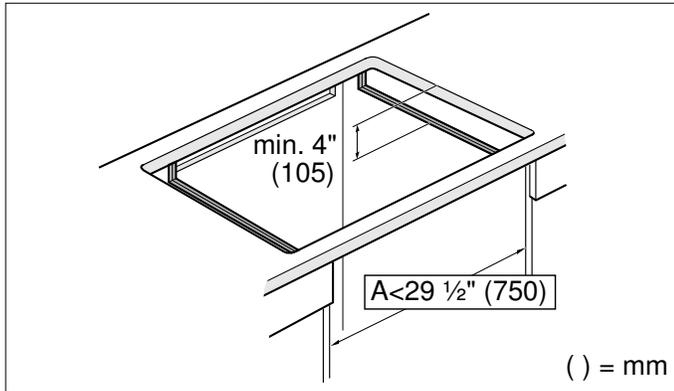
**Note:** If the appliance is installed in an island unit or another installation that is not described here, you must ensure that the cooktop is sufficiently ventilated.
