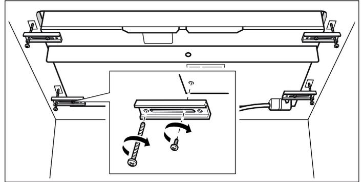
The appliance must be secured from below using the hold-down brackets provided, so it does not slip.
