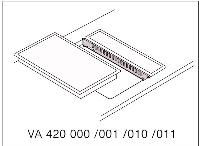
Appliances can also be installed in individual cut-outs, bearing in mind a minimum distance between the devices of 2" (51 mm).
