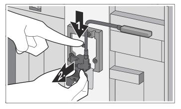
3 Detach the milk hose, dismantle the top and bottom sections of the beverage dispenser.
