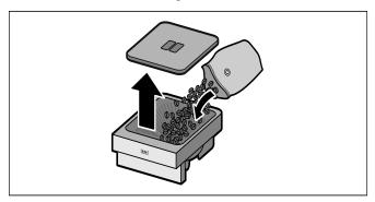
**Note:** Coffee beans that have been glazed, caramelized, or that contain other sugary additives block the brewing unit. Only use pure bean mixtures that are suitable for use in fully automatic espresso machines.
