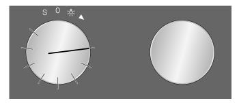
2 Use the > symbol to select the desired beverage, capacity, strength, temperature and coffee-milk ratio and use the rotary selector to save the settings.
