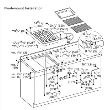
$^\star$  With appliance cover or adjustment strip. See separate planning notes on page 87. \*\* 4 1/4" (108) in the area of the cable clip (right, center).
