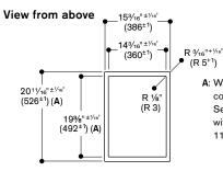
A: When installing with appliance cover consider the deeper cut-out See separate notes "assembly with appliance cover" on page 113).
