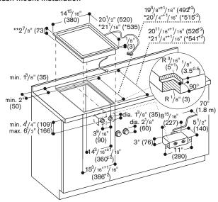
$^{\star}$  With appliance cover or adjustment strip. See separate planning notes on page 87.  $^{\star\star}$  31/2"(88) in the area of the cable clip (right, center).
