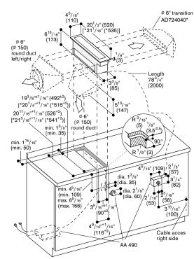
\*With adjustment strip Round duct connection, bottom Round duct connection left/right
