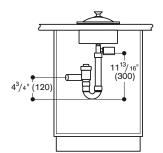
Installation possible with a direct water connection by a plumbing professional. Drainage connection in the base cabinet: For a fixed connection without free fall tube, it is necessary to install a non-return valve.
