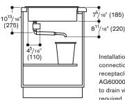
Installation possible without a direct water connection. Drainage into a water-collecting receptacle (e.g. bucket). Only possible with AG600000 drain installation set. Access to drain via a door in the base cabinet is required.
