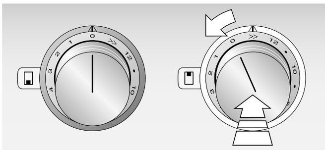
**Turning off:** Turn control knob to any other heat level. The >> symbol goes out on the cooking zone display.
