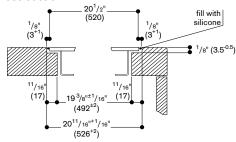
When installing with appliance cover, pay attention to the deeper cut-out and the front and rear groove width.
