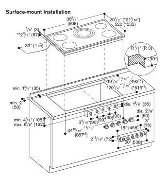
\* with adjustment strip. See separate planning notes on page 87. \*\* 3%/6"(93) in the area of the wire connection (rear, right).
