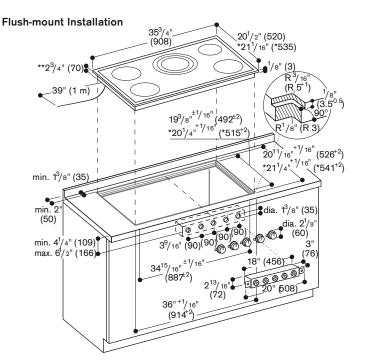
\* with adjustment strip. See separate planning notes on page 87. \*\* 3  $1 M_{10}$  (93) in the area of the wire connection (rear, right).
