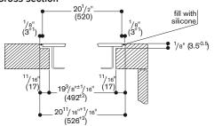
When installating with appliance cover or adjustment strip, pay attention to the deeper cut-out and the front and rear groove width.
