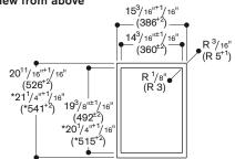
\* with appliance cover or adjustment strip (observe the front and rear asymmetrical support, see separate notes "Installation with appliance cover/adjustment strip" on page 87).
