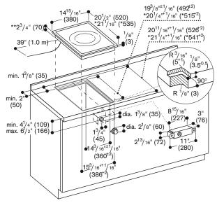
$^*$  with adjustment strip. See separate planning notes on page 87.  $^{**}$  3  $^{11}\!/_{16}"$ (93) in the area of the wire connection (rear, right).
