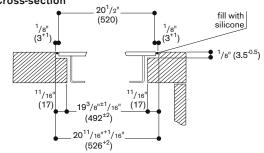
When installing with appliance cover or adjustment strip, pay attention to the deeper cut-out and the front and rear groove width.
