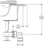
\*  $2^{1}/16^{\circ}$  (53 mm) with appliance cover or adjustment strip.
