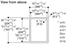
\* with appliance cover or adjustment strip (observe front and rear asymmetrical assembly. See separate notes "assembly with appliance cover/adjustment strip" on page 89).
