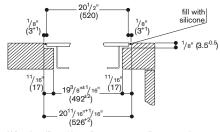
When installing with appliance cover or adjustment strip, pay attention to the deeper cut-out and the front and rear groove.
