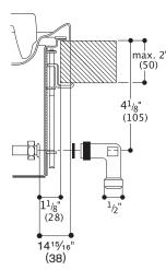
Note: When planning installation over an oven, plan gas connections and shut-off in adjacent cabinet.
