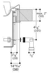
Note: When planning installation over an oven, plan gas connections and shut-off in adjacent cabinet.
