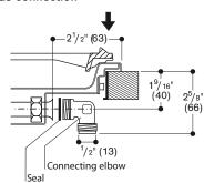
Note: When planning installation over an oven, plan gas connections and shut-off in adjacent cabinet.
