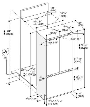
The door face dimensions are designed for a maximum gap of % " (3 mm). See more details on page 247.
