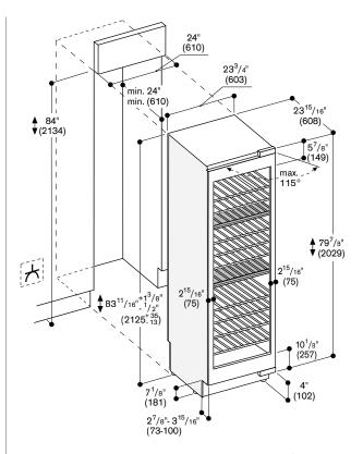
The door face dimensions are designed for a maximum gap of 1/s" (3 mm).
