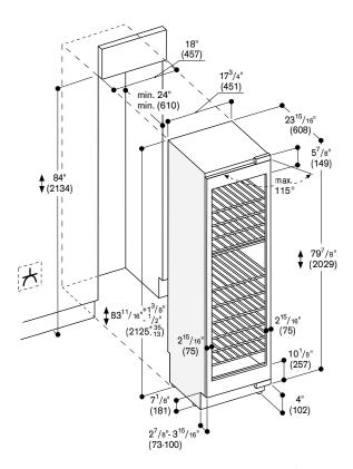
The door face dimensions are designed for a maximum gap of ½" (3 mm).
