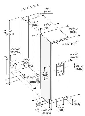
The door face dimensions are designed for a maximum gap of 1/8" (3 mm). \* For a flush-mounted appearance, the minimum cut-out depth must be 25". See more details on pages 170 and 177.
