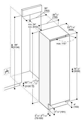
The door face dimensions are designed for a maximum gap of  $\,\%''$  (3 mm). See more details on page 247.
