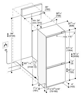
The door face dimensions are designed for a maximum gap of  $\mbox{1/6}^{"}$  (3 mm). See more details on page 247.
