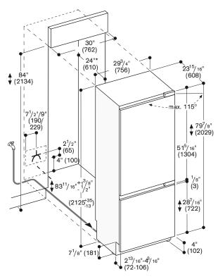
The door face dimensions are designed for a maximum gap of  $1\!/\!\!s"$  (3 mm).
