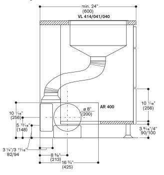
Connecting Vario 400/200 series VL downdraft to AR 413 recirculation kit using  $\emptyset$  5" flexible duct
